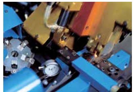
Stelliting with resistance welding process
