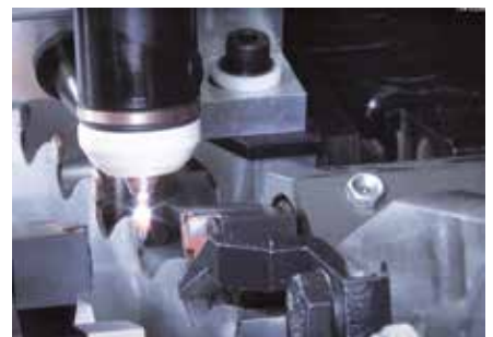
Stelliting with plasma welding process
