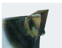
Stellited tooth in resistance welding process
