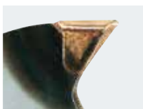
Stellited tooth in plasma welding process
