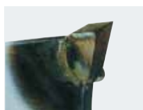
Stellited tooth in resistance welding process
