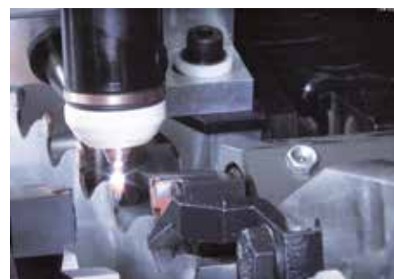
Stelliting with plasma welding process
