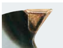
Stellited tooth in plasma welding process
