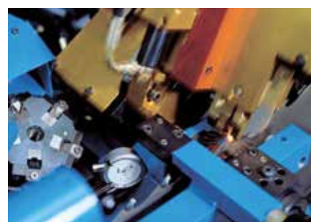
Stelliting with resistance welding process
