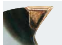
Stellited tooth in plasma welding process
